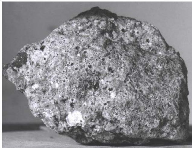
Figure 1: Photo of 60625 showing zap pits all sides. NASA S72-44915. Sample is 5 cm across.
