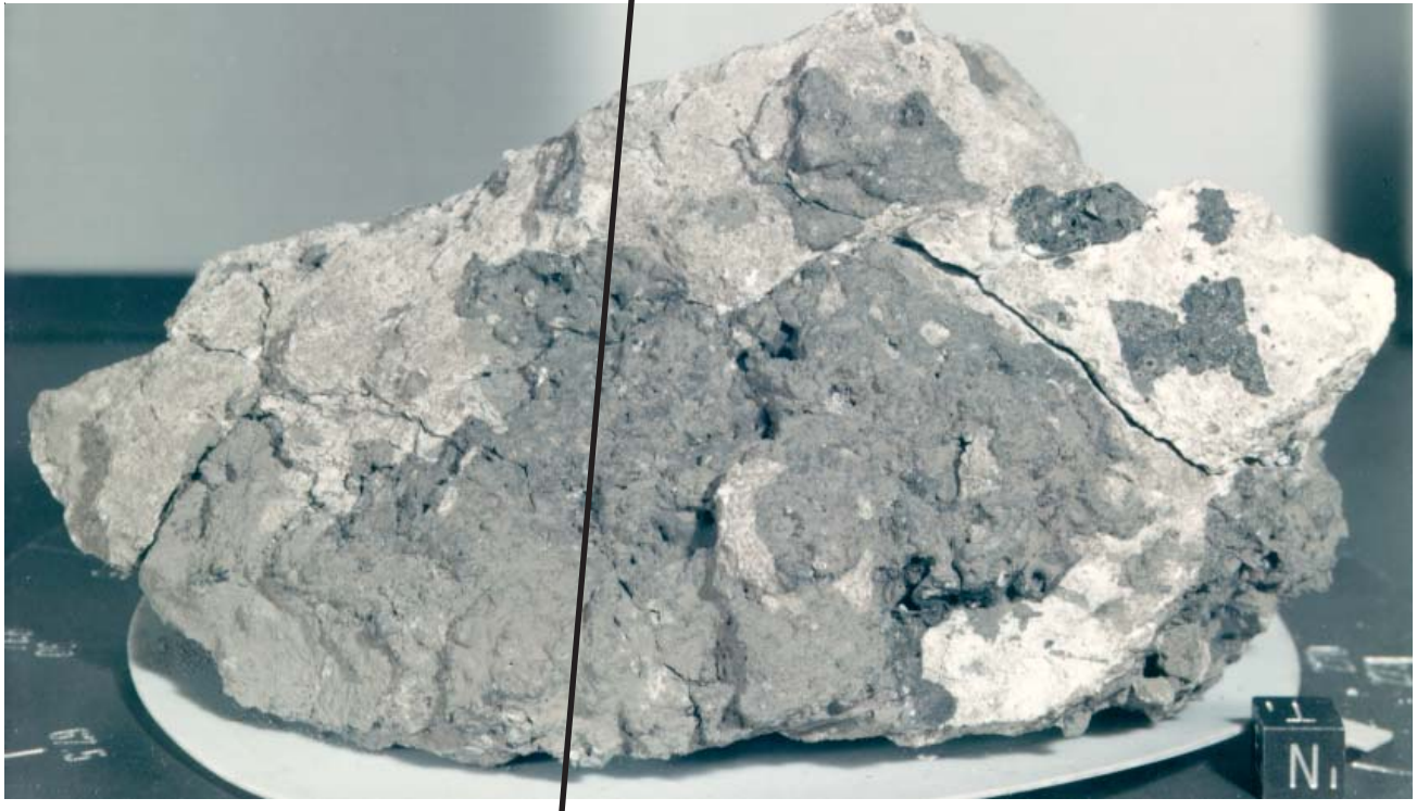
Figure 1: Photo of 62255 showing glass splash on anorthosite. Cube is 1 cm. NASA S # S72-38309.
