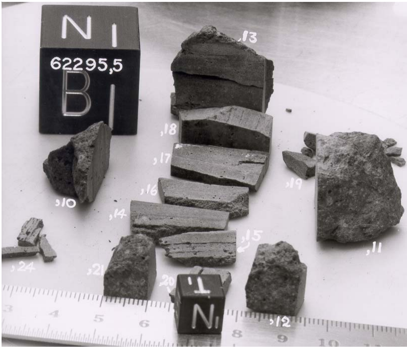
Figure 17: Exploded parts diagram for 62295,5. NASA S72-50654. Large cube is 1 inch.
