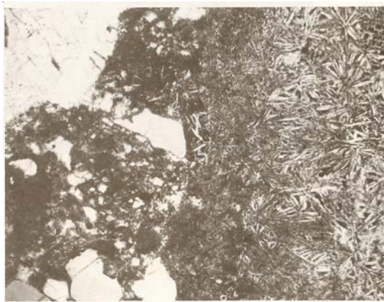
Figure 3: Portions of 63538 have devitrified glass.
