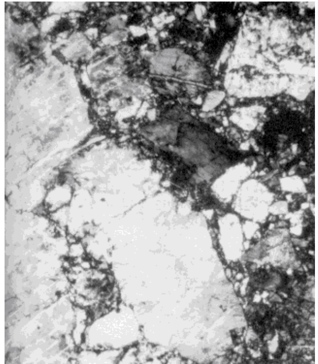
Figure 6: Photomicrograph of thin section 65035,8 showing coarse plagioclase in anorthosite portion. Crossed polarizers. Field of view 2 mm. From Ryder and Norman 1980.
