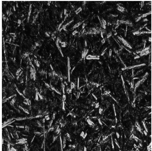
Figure 8: Thin section photomicrograph of melt in 66055.
