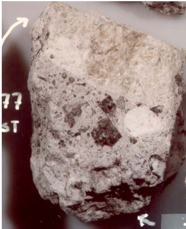
Figure 4: Photo of clasts and matrix in 67016,277. NASA # S82-27849. Size of clast is about 1.5 cm. Bother light and dark clasts are included in light grey matrix.
