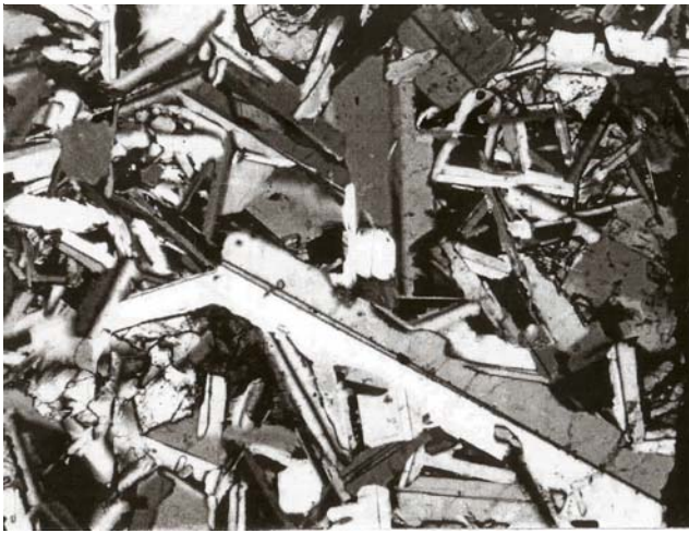
Figure 2 a: Internal texture of 68559,1 (Ryder and Norman 1980). Crossed polarizer - width of field is 2 mm.
