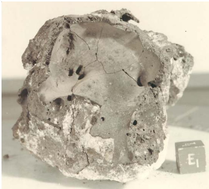
Figure 2: Back side of 68515 showing glass coating. S72-43452
