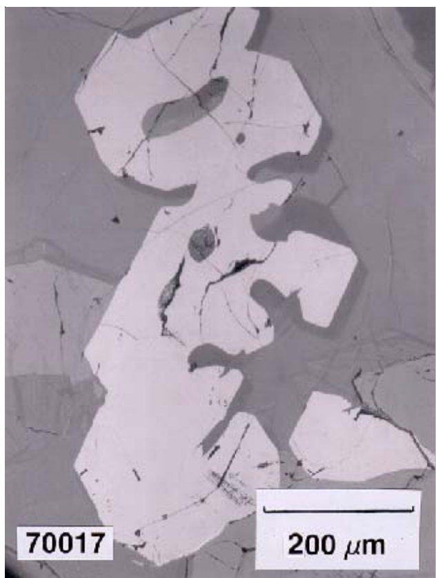
Figure 5: Reflected light photo of polished thin section illustrating habit of ilmenite in 70017.
