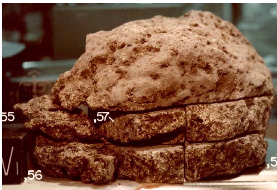
Figure 11: Additional saw cuts of 70035 made in 1981 (see flow diagram). Note glass coating in this side. NASA S81-27729. Cube is 1 inch.
