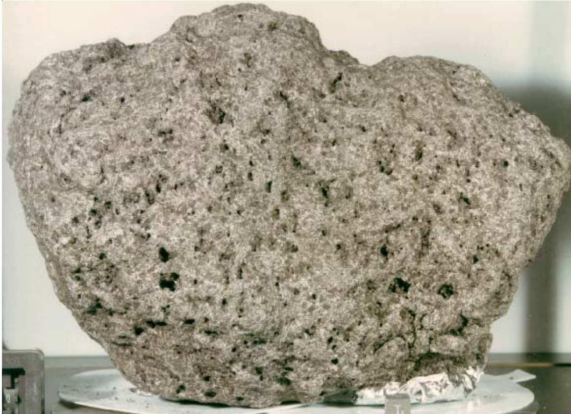
Figure 1: Photograph of top surface of 70035 illustrating vugs and vesicles. Note the smooth, rounded surface shaped by micrometeorite bombardment. Small cube is 1 cm. NASA photo # S72-56385.
