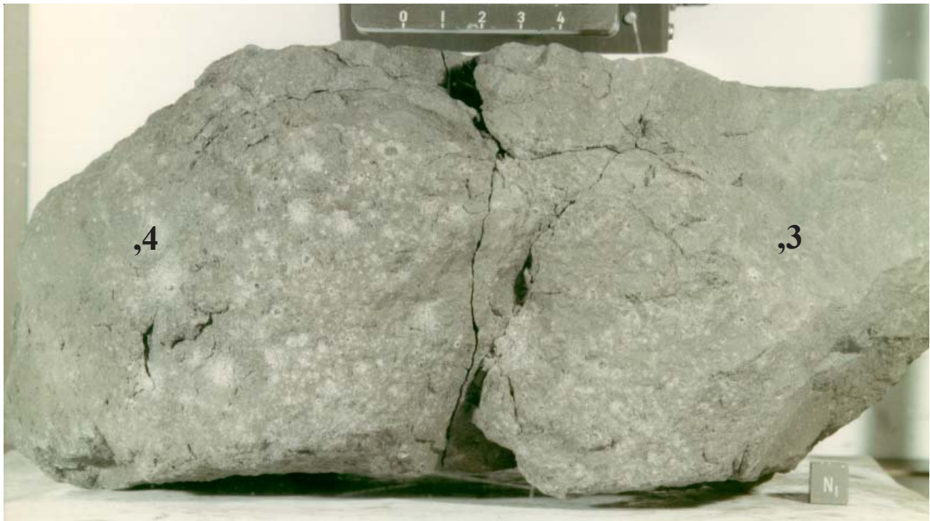
Figure 15: Photo of 70215 illustrating zap pits. Scale and cube are in cm. NASA photo # S73-15710.
