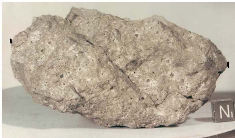
Figure 2: Photo of 72355 with numerous zap pits. Cube is 1 cm. S73-15355.
