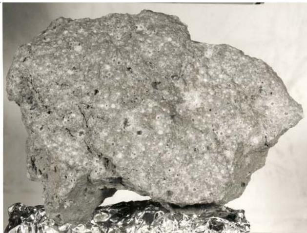
Figure 2: Photo of exterior surface of 72395 showing numerous zap pits. Sample is about 10 cm. S73-23979.
