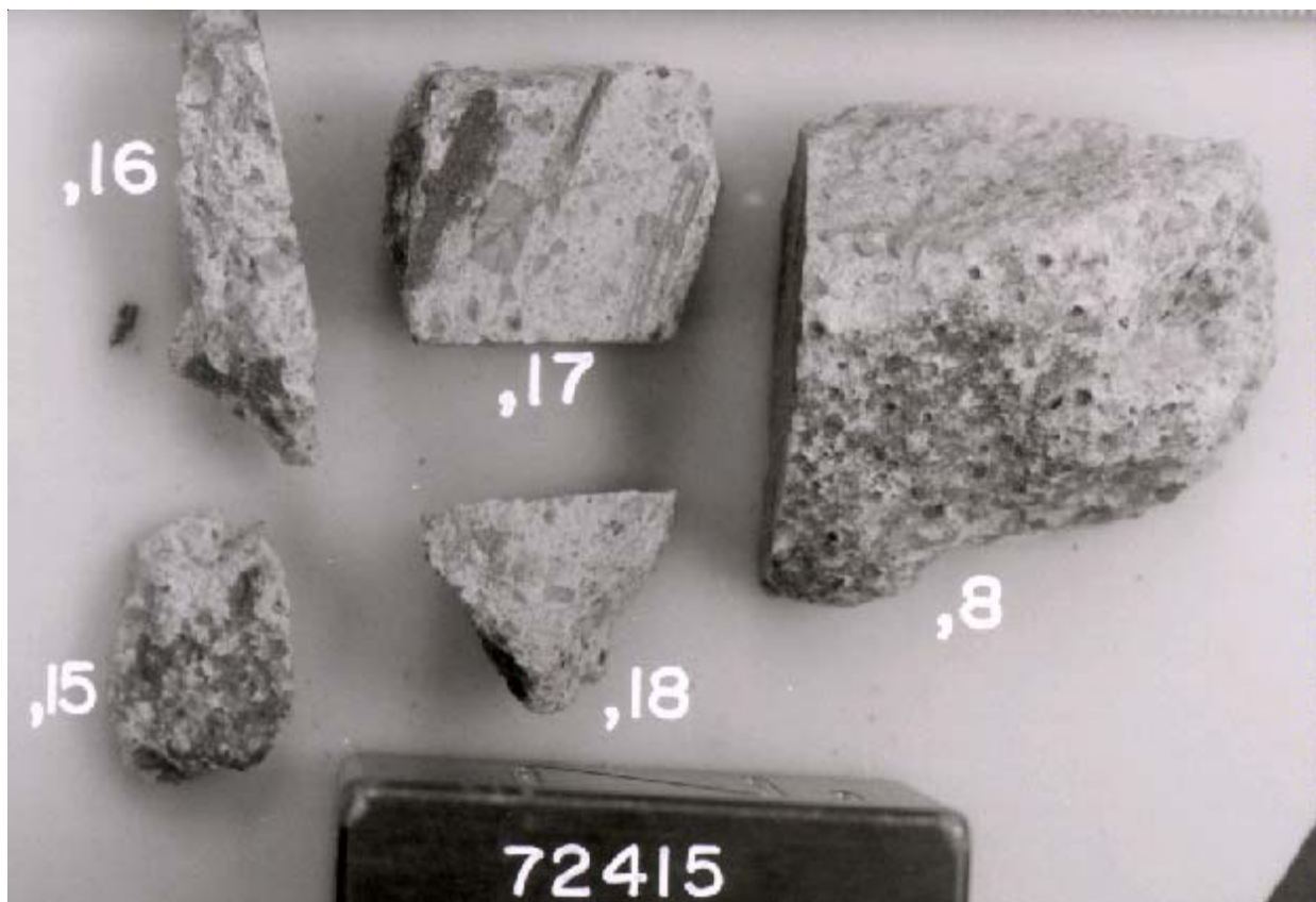
Figure 11: The largest piece of 72415 was sawn to produce a slab (,18 and ,17). Edge of cube is 1 inch. NASA# S74-19014.
