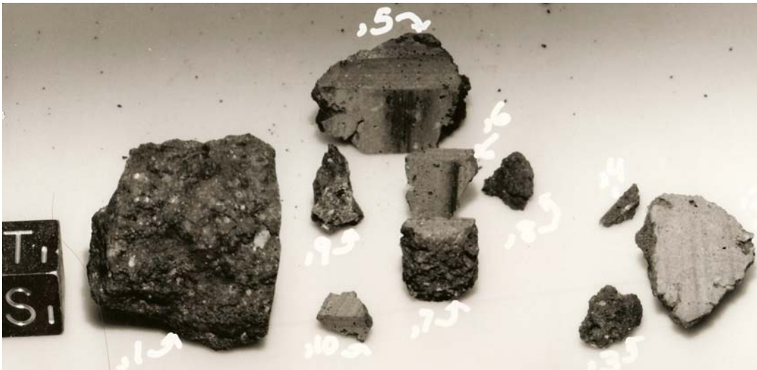
Figure 4: Photo of 72738 after cutting slab. S74-20182. Cube is 1 cm.
