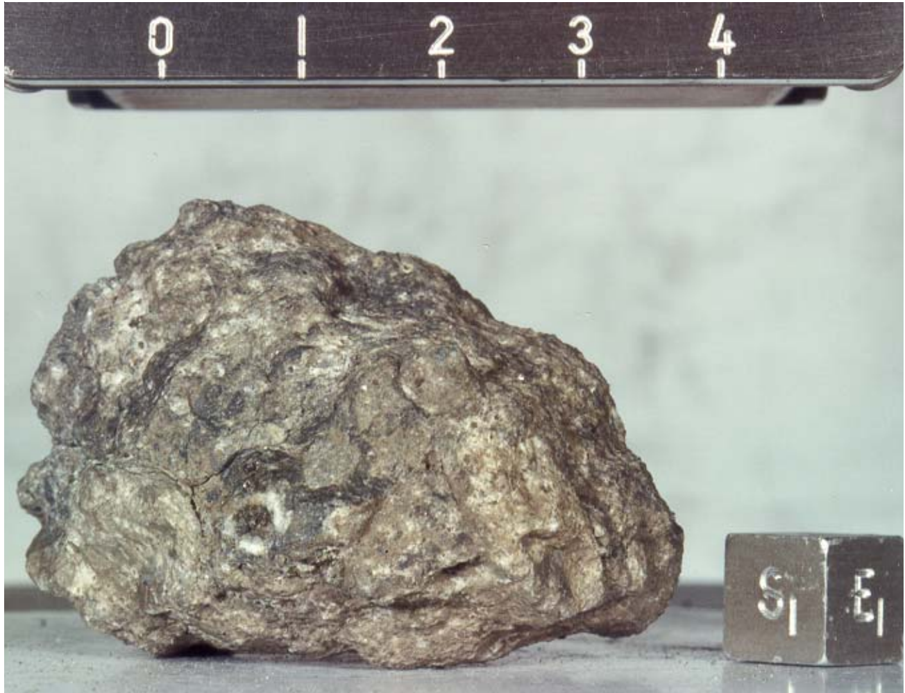
Figure 1: Photo of 73155 showing micrometeorite crater with spall zone. NASA S73-23887. Cube and scale are 1 cm.
