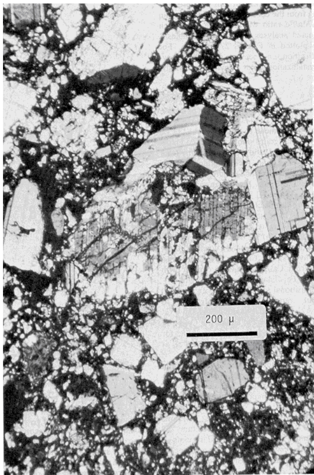
Figure 3: Photomicrograph of "gabbroic" lithic clast in crushed matrix of 73217 (from Ishii et al. 1983).
