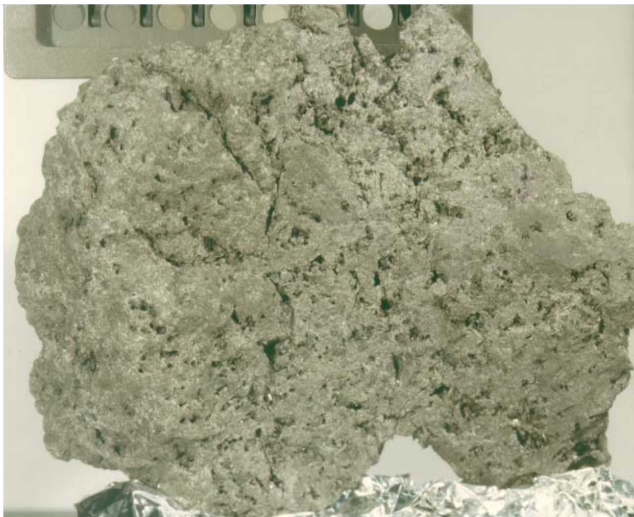
Figure 1: Photo of vuggy mare basalt sample 75075. NASA S73-15337. Sample is about 12 cm across.
