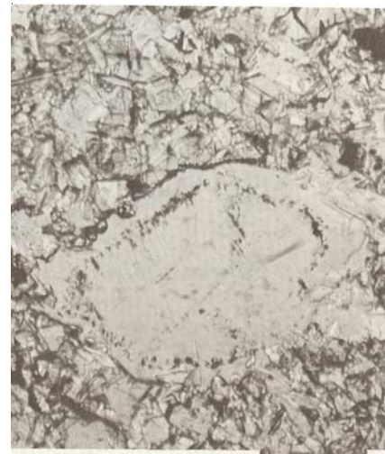
Figure 4: Plagioclase clast with necklace and overgrowth. Field of view 0.5 mm. (from McGee et al. 1977)
