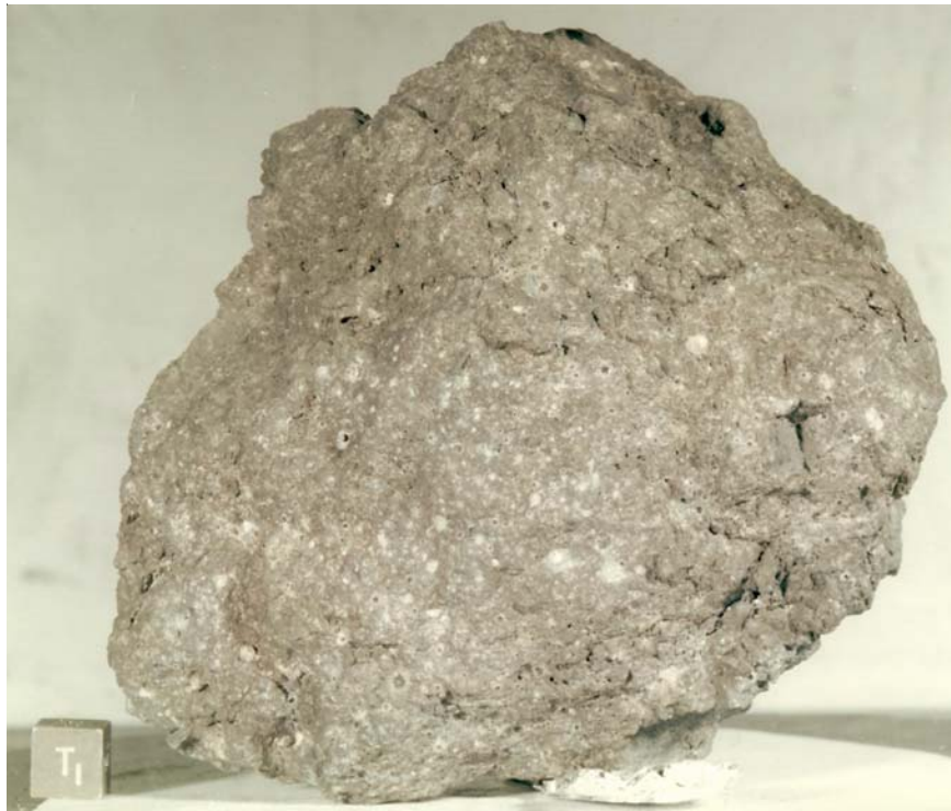
Figure 2: Photo of front, exposed, surface of 76315. The lack of zap pits on the upper left corner, indicate that this corner was facing down on the boulder. Cube is 1 cm. S73-17108.
