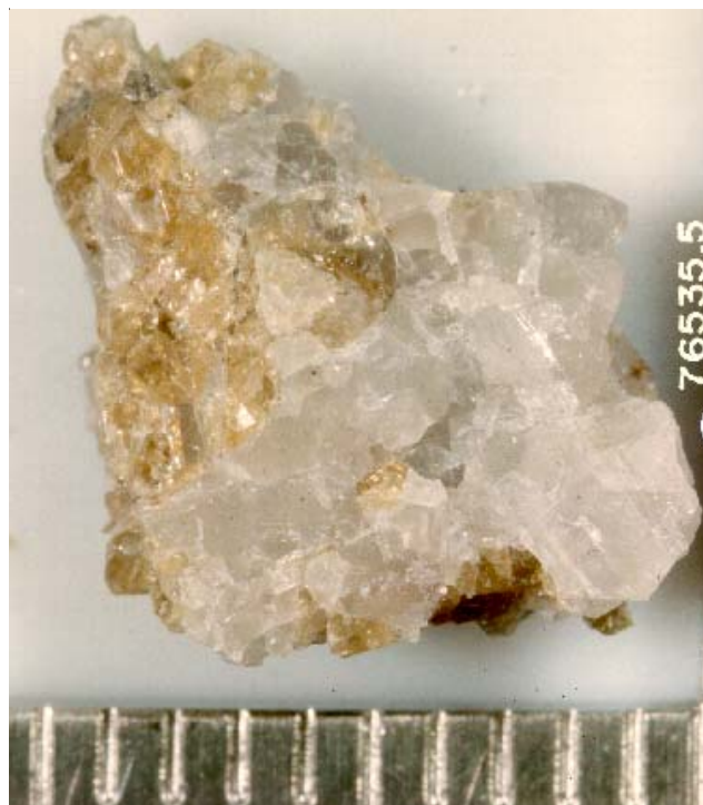
Figure 2: Photograph of small piece of 76535 (scale in mm). Note striations on plagioclase. Photo # S-73-19614
