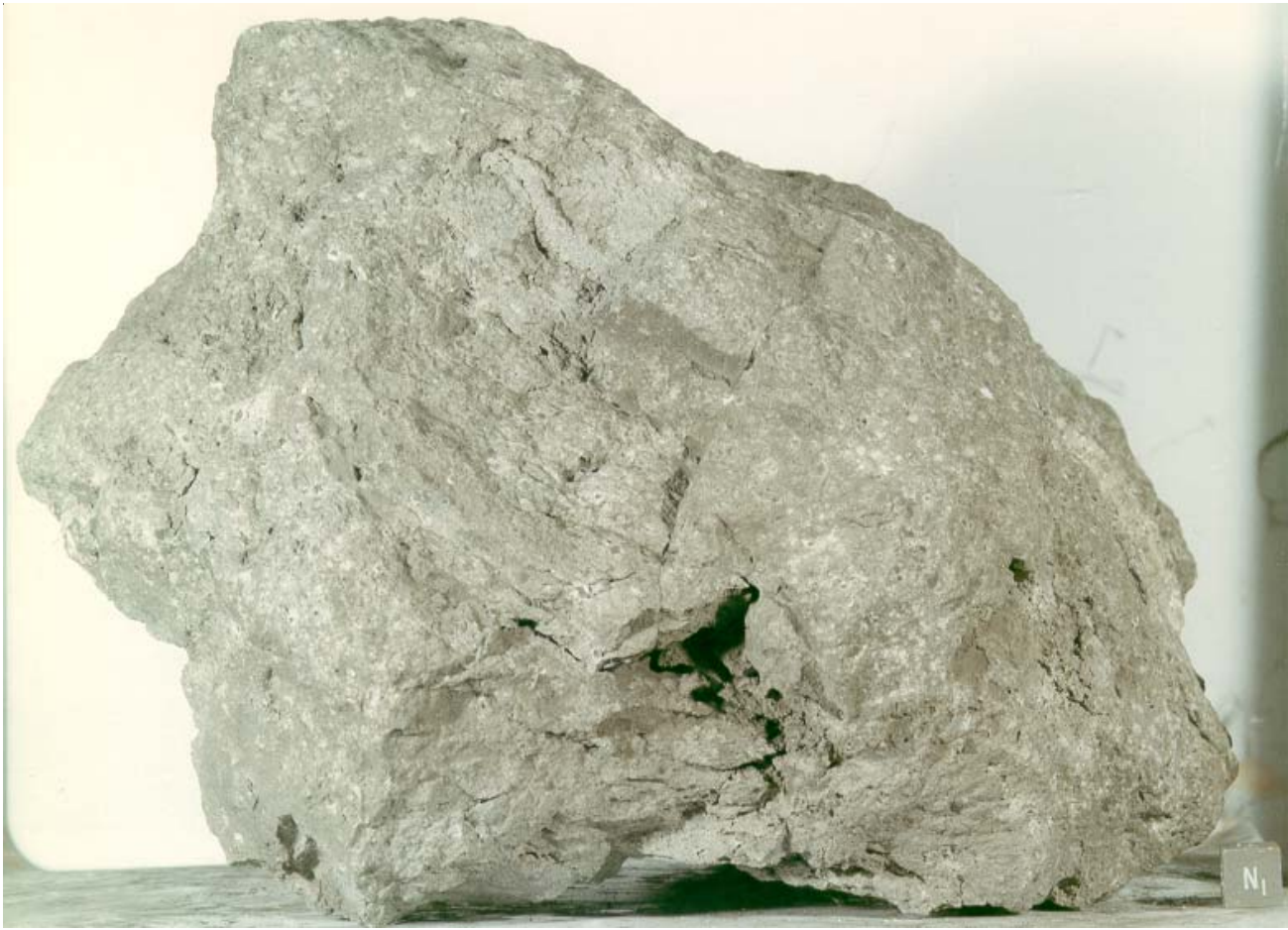
Figure 3: PET photo of 77035 showing banded structure and void space. NASA S73-15904. Cube is 1 cm.
