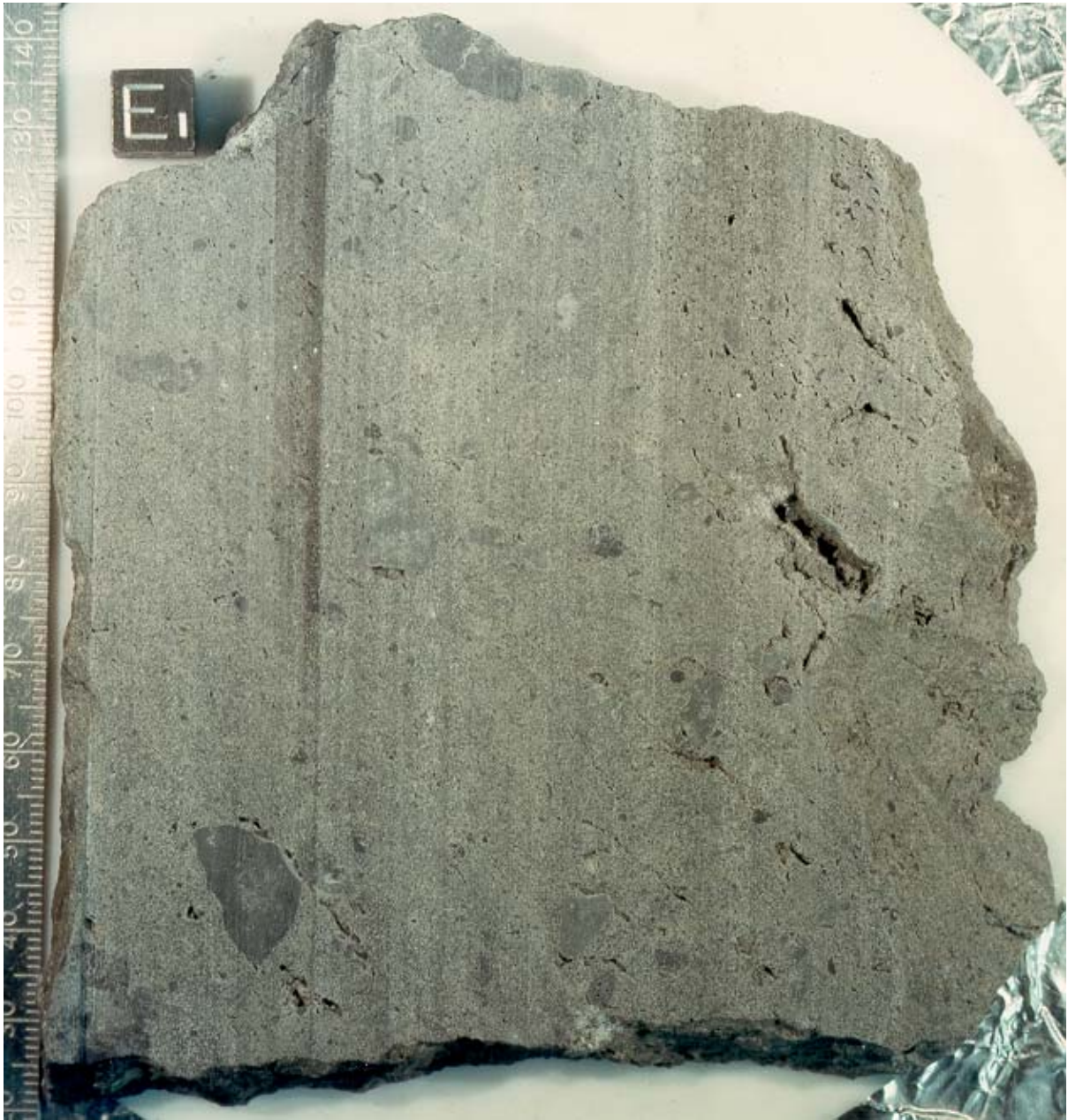
Figure 13: Sawn surface of 77035,155 showing dark aphanitic clasts in foliated matrix (see also figure 2). NASA S90-28807. Cube is 1 cm.
