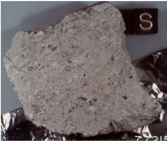
Figure 2: Sawn surface of 77215,16 showing relict igneous texture. NASA photo # S83-34595. One cm cube for scale.
