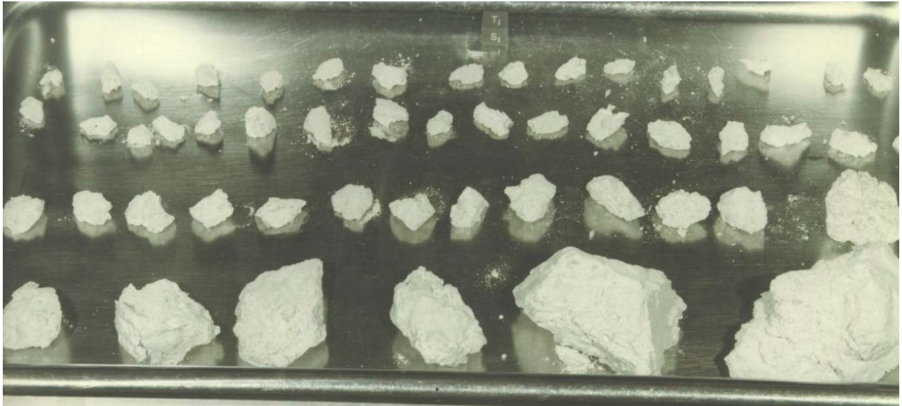
Figure 1: Tray full of pieces of 78155. Largest piece is about 7 cm. Small pieces and cube are 1 cm. NASA S73-15407
