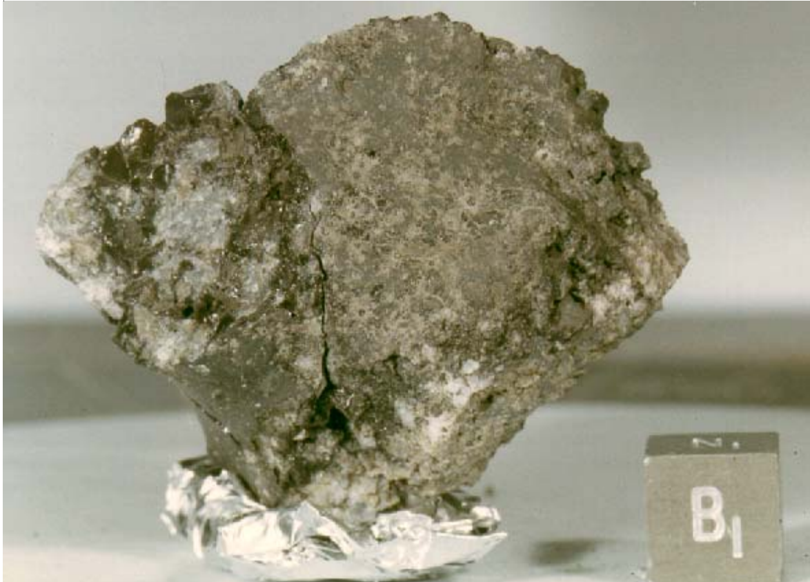
Figure 1: PET photo of 78255 showing relict zap pits on underside of boulder. Cube is 1 cm. Photo # S73-15190
