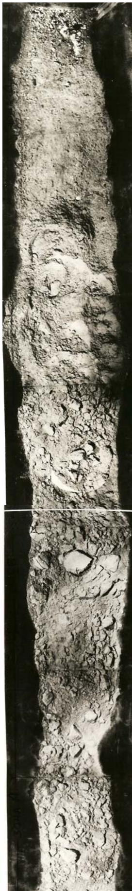
Figure 1: Copy of Russian photo of Luna 16 core after initial dissection showing position of three samples provided to US workers (21000, 21010 and basalt chip B 21020). NASA S71-38646 and 38647). Location of B is approx. See also figure 9.
