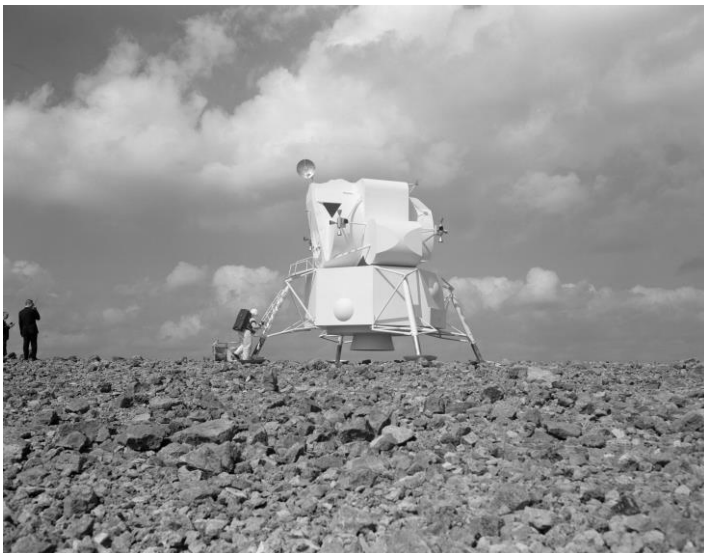
Figure 5. The "Rock Pile" being used in a test of a suited subject practicing ascent and descent from the lunar module. (NASA photo S65-22083)
