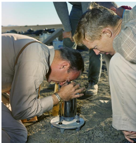
Figure 30. Astronauts Ed Mitchell and Stuart Roosa learn to use a gravity meter on a geology trip to the Pinacates volcanic region of Sonora, Mexico, in November 1966. (NASA photo S66-65992)
