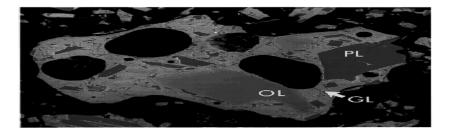
Figure 1. JSC-1 grains in polished section. Phases include glass (GL), plagioclase (PL) and olivine (OL). SEM back-scattered electron image. Frame width =  $520 \, \mu m$ .
