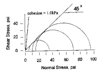
Figure 4. Mohr stress circles used to determine angle of internal friction (45°) and cohesion (1.0 kPa) for JSC-1.
