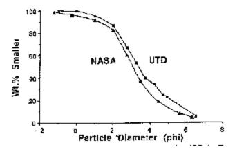
Figure 3. Particle size distribution curves for JSC-1. Particle diameters in phi units ( $^- = - (\ln d) / (\ln 2)$ , d = diameter in mm).
