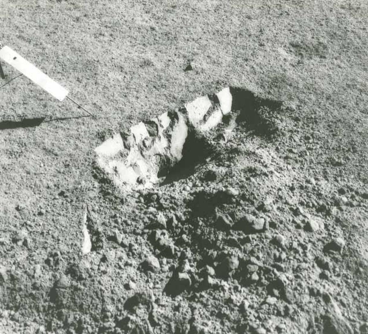
**Fig. 7:** This is a shallow trench dug by an Astronaut on Apollo 17. The smooth, nearly vertical wall is due to the cohesion and frictional shear strength of the lunar soil.
