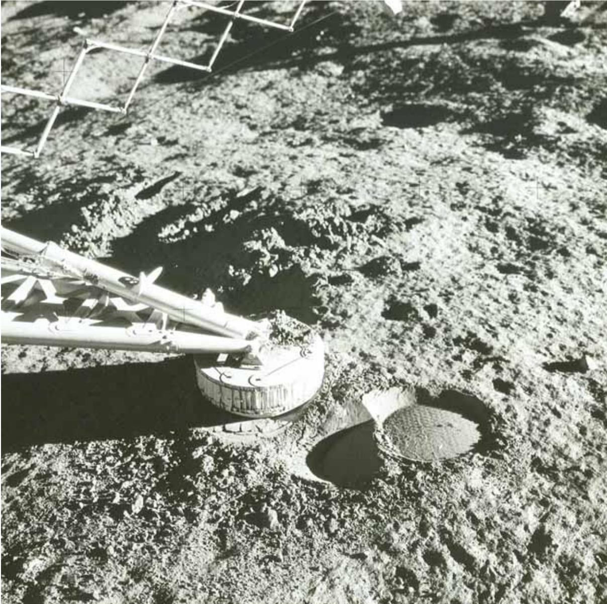
**Fig. 6:** When Surveyor III landed on the Moon, it bounced a couple of times. The fine, delicate “honeycomb” pattern on the bottom of one of the footpads was preserved in the cohesive lunar soil, as shown in the lower right-hand corner of this Apollo 12 photograph.
