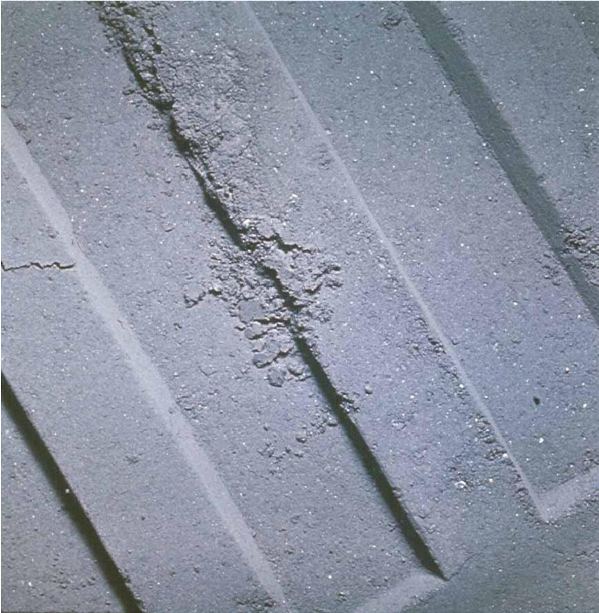
**Fig. 5:** This is a closeup of an Astronaut footprint taken on Apollo 12. It is one-half of a stereo pair. The field of view is approximately 50 mm × 50 mm. Note the cohesiveness of the lunar soil.
