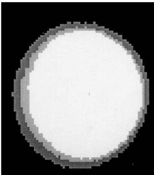
Fig.1. The image of the Moon was transmitted by satellite GOMS on March 3, 1995 in the working infrared range 10.5 - 12.5-micron. The phase angle of the Moon is  $-26.5^\circ$ . The isotherms for IR radiation temperature of the lunar surface are the system of concentric circles, which has centre in sub solar point (longitude, 21.33E, latitude, 1.13N). The centre of the apparent disk has coordinates: longitude, 5.69W, latitude, 6.29N. The lunar surface has radiation temperature 397.0 K - 261.1 K.
