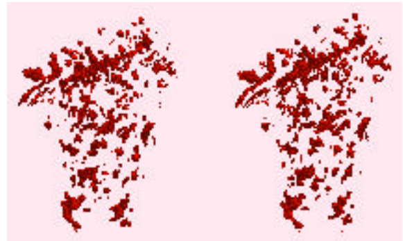
Fig.3. A stereo graph showing chromite distribution. The voxels of cm in Fig.2(right) are presented.
