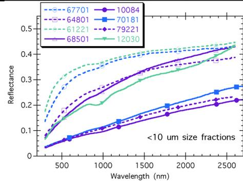
Figure 4. Reflectance spectra of  $<10\mu\text{m}$  size fraction of lunar soils (see table). Wet sieved = dotted line, dry = solid. More mature = darker line.
