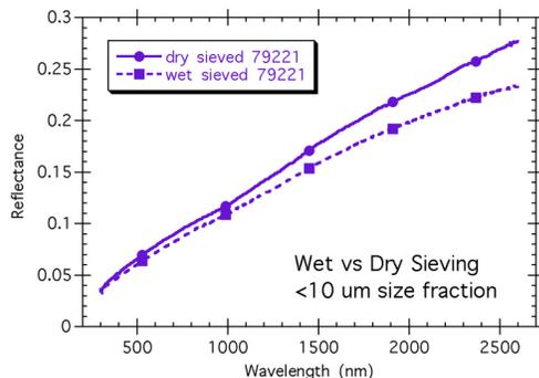
Figure 3. Reflectance spectra of lunar soil 79221  $<10\mu\text{m}$  processed in 2 ways [6,9]
