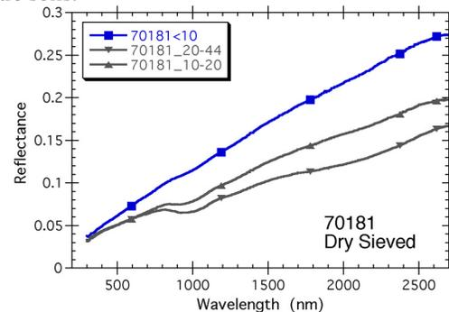
Figure 2. Size fractions from a basaltic soil [6]. Sample prepared by dry sieving with a sonic sifter.
