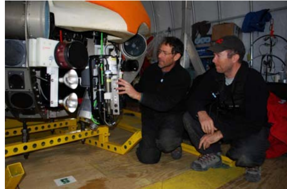
Figure 1: Science package that is lowered through the water column while the vehicle holds station under the ice cover
