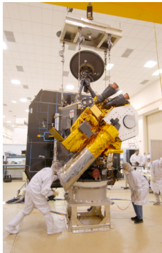
Fig.1. The Deep Impact Flyby spacecraft carries two imagers (MRI and HRI) and an IR spectrometer.
