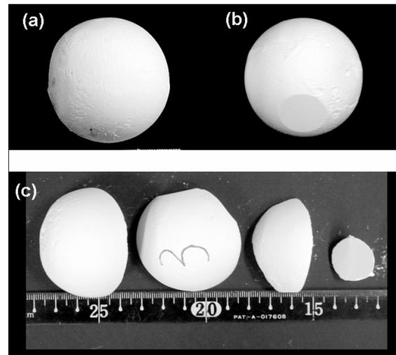
Fig. 1 Porous gypsum targets. (a) Original, (b) compacted, and (c) fragmented spheres of 50 mm in diameter. The impact velocities were (b) 10.2 m/s and (c) 22 m/s.
