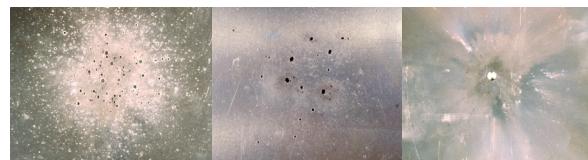
Figure 2: Witness plates of disrupted impacting Pyrex projectiles under increasing atmospheric pressures. Under vacuum, the shattered fragments create a dispersed debris cloud (left). At 170mm argon, however, interacting shocks spread fragments apart (center). At high atmospheric pressures (700mm argon), a single hole corresponding to the assemblage of particles contained by the mach cone.
