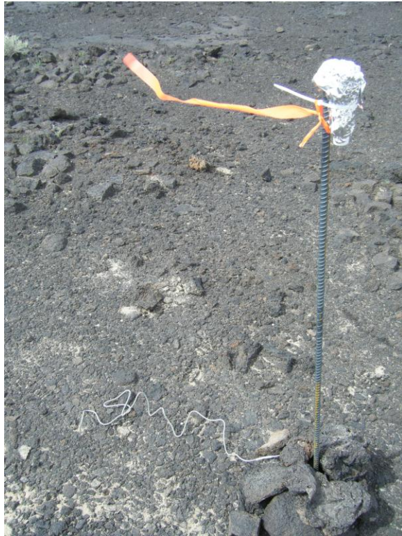
Figure 2: Sensor arrangement to measure rock surface, cairn, and air temperatures.
