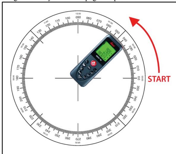
Figure 1: Laser disto and protractor plate.
