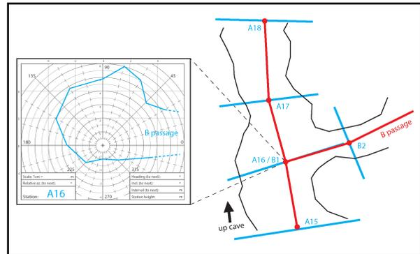
Figure 2: Sample cross-section and line plot.
