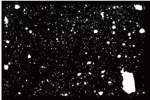
Figure 2. Slide scanner image of a 7- \mu\text{m} thick foil from detector 3 of shot 011015. The image resolution is 2700 dpi.
