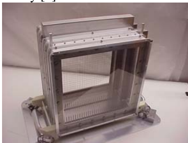
Fig. 1 Lab set-up of the dust trajectory sensor
