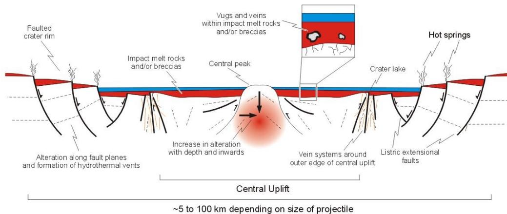
**Figure 1.** Schematic cross-section showing the distribution and style of hydrothermal alteration expected for complex impact structures on Mars.
