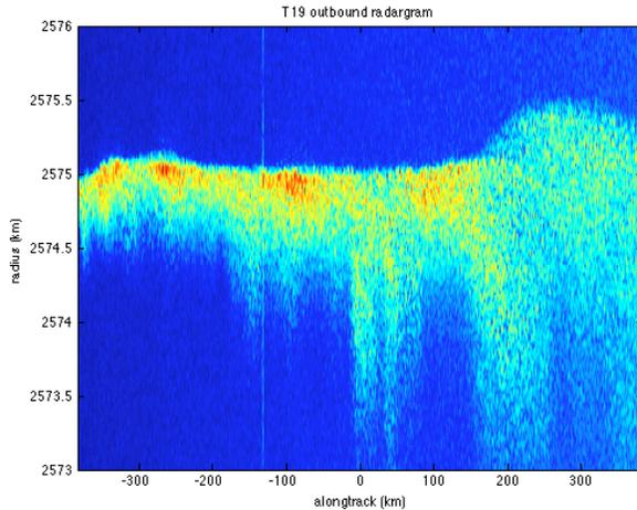
*Figure 1: Radargram of T19 altimetry : Red represents strongest signal while the width is related to the surface properties such as material and slope. The spacecraft altitude varies from about 4000 km on the left to 10,000 on the right.*
