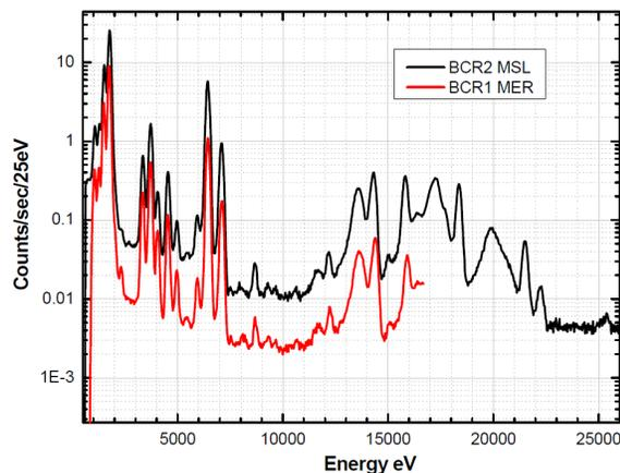
**Figure 4:** Comparison of fluorescence signal response employing the MER (red) and MSL (black) versions of APXS for the same integration time.
