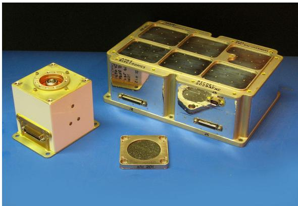
**Figure 1:** MSL APXS flight instrument. The sensor head (left), mounted on the MSL robotic arm; the electronics box (back right), located inside the rover, contains a microcontroller to process the analogue signals and to command the instrument; the basaltic calibration target (center).
