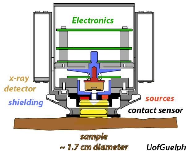
**Figure 2:** Sketch of the new APXS sensor head geometry. The opening of the JPL provided contact sensor plate is wide enough to measure either in contact or with a standoff.
