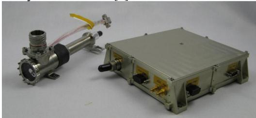
Fig. 4. MOMA laserhead (left) and laser electronics and pump module (right).
