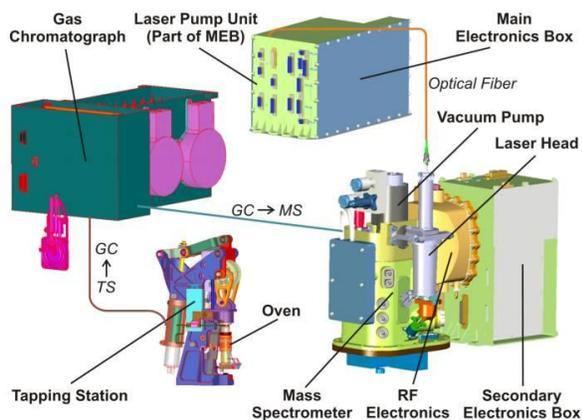
Fig. 1. Overview of MOMA instrument modules (not to scale).
