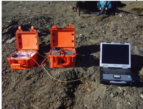
Fig. 6. MOMA GC breadboard during AMASE fieldtrip.
