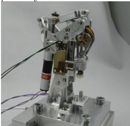
Fig.5. Tapping station prototype on pressure test stand.
