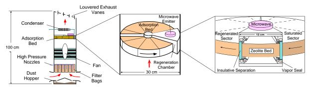
Fig. 2. Water Vapor Adsorption Reactor.
