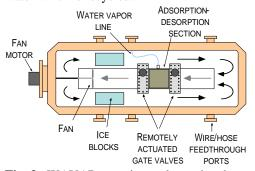
Fig. 3. WAVAR experimental test chamber.
