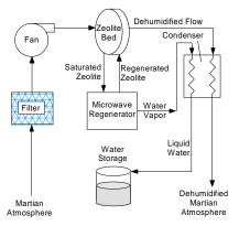
**Fig. 1.** Process schematic of WAVAR, the Water Vapor Adsorption Reactor.
