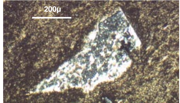
Fig 12 checkerboard texture in feldspar
