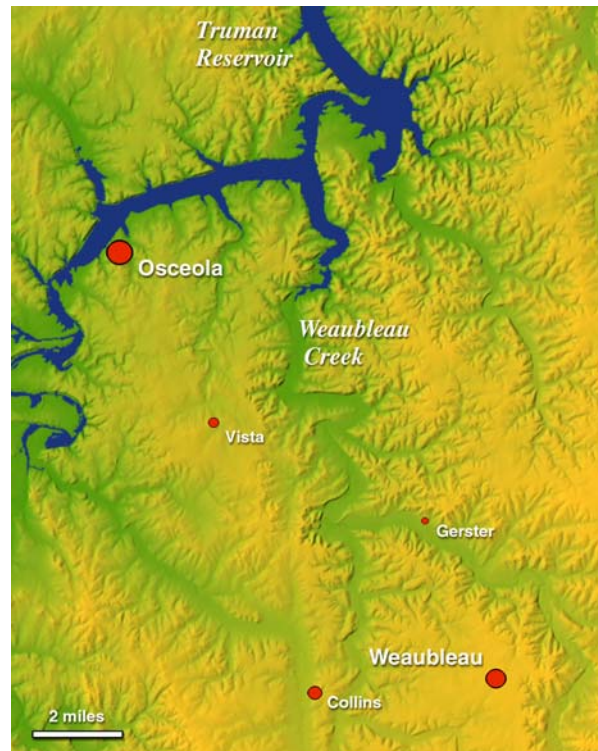
Figure 1. Digital elevation model of the Weaubleau-Osceola structure shows a relict circular depression that outlines the transient crater. Although the uppermost target rocks are Mississippian carbonates, uplifted areas of Lower Ordovician dolomite that we interpret as relict parts of the crater flank the southwestern and northeastern margins and are beveled below the sub-Pennsylvanian unconformity.
