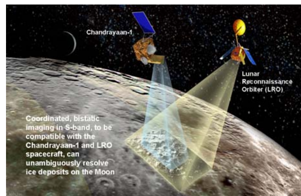
Fig.1 Coordinated bistatic imaging of the lunar poles can unambiguously map lunar ice deposits.
