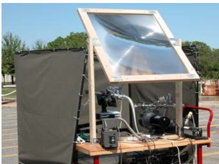
Figure 1. The prototype setup with the Fresnel lens.
